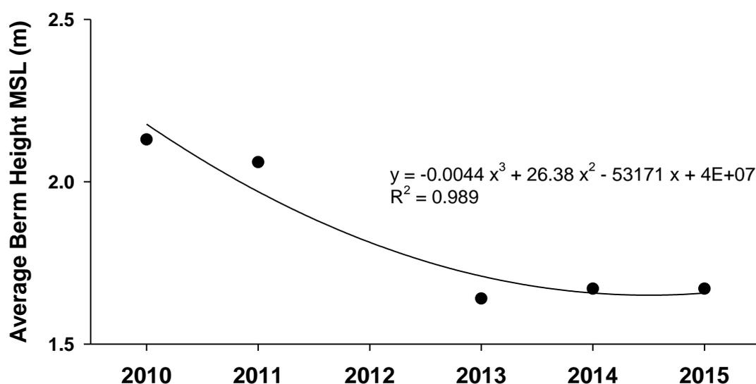
**Figure 8** Average berm height (m) above MSL across the mouth of the Seekoei Estuary between 2010 and 2015 inclusive. Fixed points were measured monthly between two base stations asset out in Table 4.
