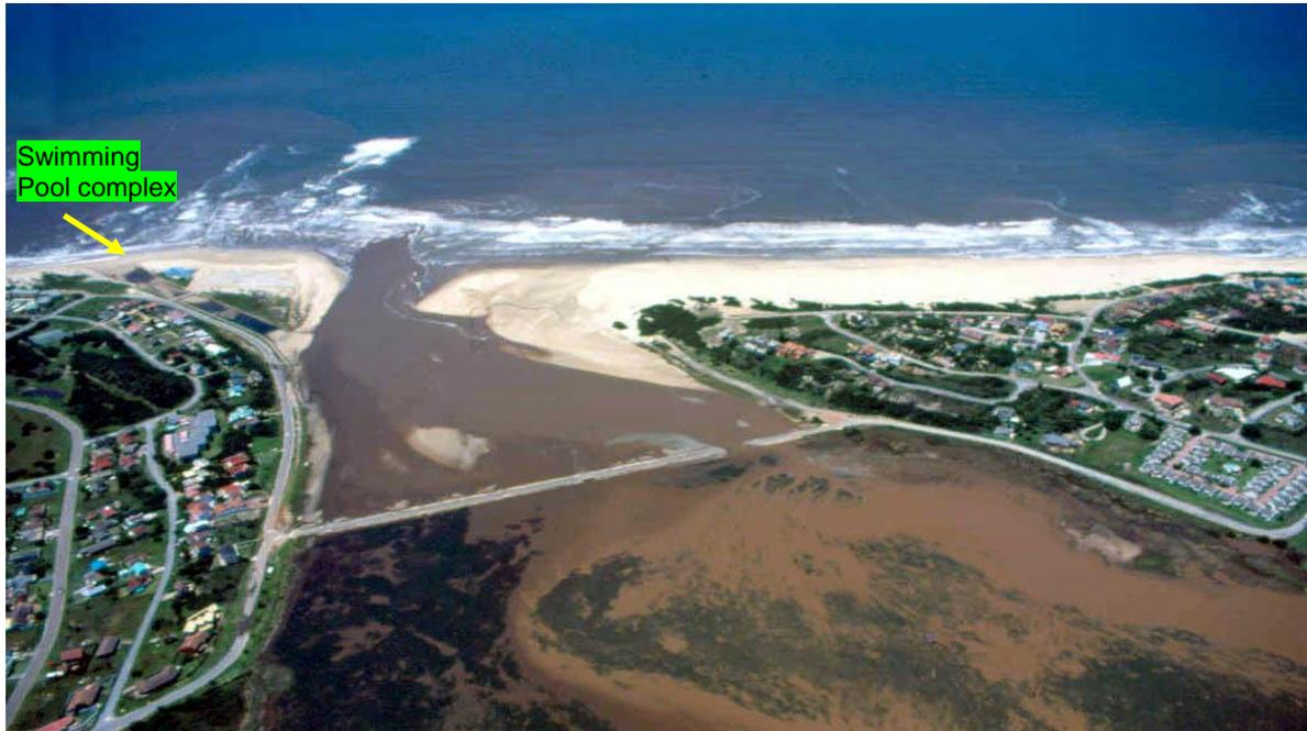
**Plate 2** At the time of this photograph (~mid 1980's), the original rubble causeway had been breached and floodwaters eroded a relatively deep and wide channel. The photograph also shows a plume of discoloured estuarine water radiating from the mouth – refer to Figure 5 (Photograph from T Wooldridge).
